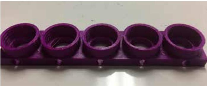
3D Printed manifold for gas collection. The .stl file for this manifold is available on the [www.kscorn.com](http://www.kscorn.com) to allow teachers to print more if needed.
