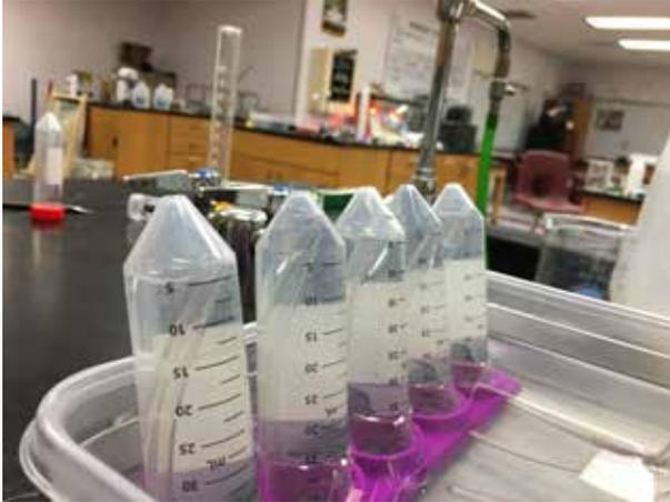
Filled manifold with tubing from samples inserted. Ready to collect any CO<sub>2</sub> gas produced.
