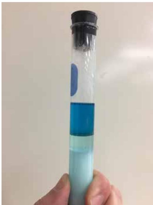
Potassium carbonate has saturated the water and forced the ethanol out of solution. The food coloring stays in the ethanol layer. This should be nearly pure ethanol.
