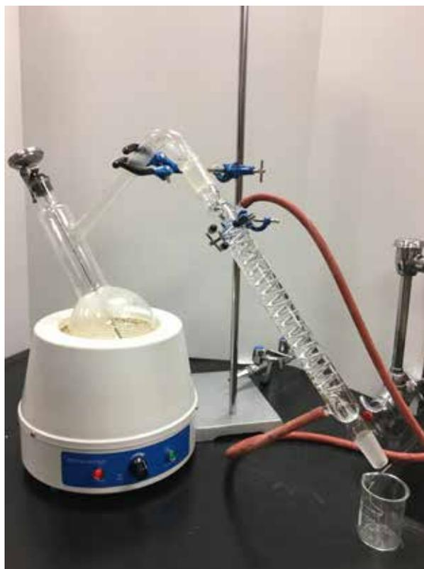
1. Set up the distillation apparatus as shown in the image above. Make sure to either grease or wet the ground glass joints before connecting them. This helps to prevent any vapor from escaping the joints and to keep the joints from freezing together.
