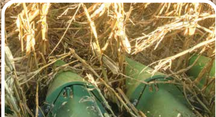
THE COMBINE'S HEADER PICKS THE CORN PLANT
